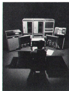
Cover: Although it could be mistaken for an organist in concert, this photo actually shows the new HP 3000 Computer System harmoniously coordinating the activities of several users—it handles multiple processing modes, users, and languages all at the same time. The panels with the red lights in the foreground are control panels used for hardware maintenance and system checkout.
